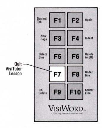
**Figure 1.** Attach the special "overlay" label over the function keys on the left side of your keyboard.
